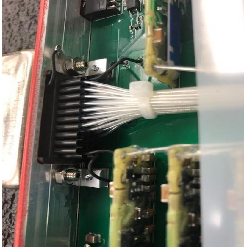
Figure 3. Slot 0 module back side of Radiall connector.
